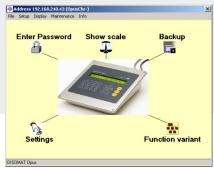
To use them, one of the 'function variants' in the instrument is activated. This puts DISOMAT into a configuration for specific applications that both allocates the essential actions to the six function keys and assigns the inputs and outputs of the instrument to the matching signals.
